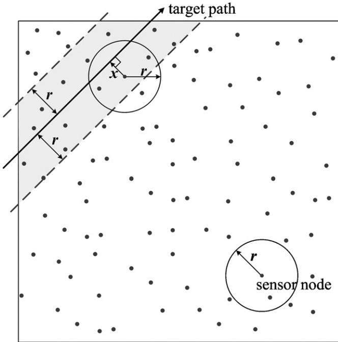
Fig. 1. Illustration of DZ and sensing area of sensor in the AoI.
