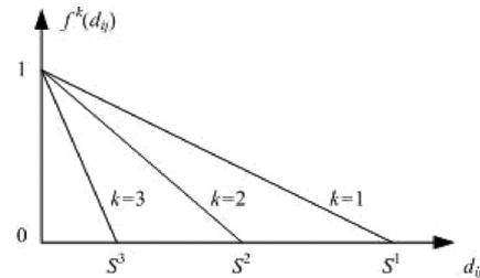
Fig. 1. An illustration of coverage function with  $K = \{1, 2, 3\}$ , where 1, 2, and 3 indicate the type I (large), type II (medium), and type III (small) facilities.
